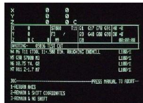
Figure 4-1 The control in waiting mode.
